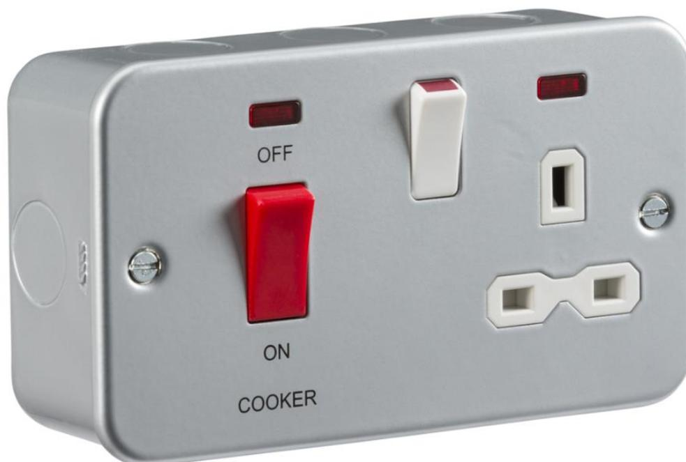
Cooker control units enable isolation of the unit so that maintenance and repairs to be carried out separately. The unit can be switched off, preventing the appliance from being turned on accidentally - for example whilst cleaning. Control two or more cooking appliances in the same room, providing rating is sufficient. This model is double sized with 45A rating with built in 13A socket and neon's
