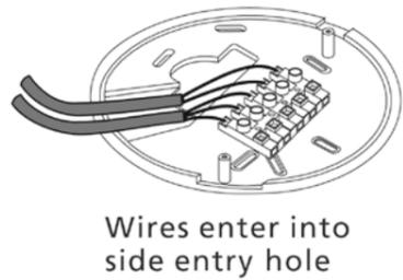
Wires enter into side entry hole
