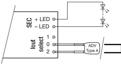
**375 mA:** Terminal 0 and 2 connected with resistor ADV Plug Type B BR (article number: 28001772)
