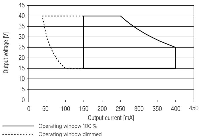
Make sure that the LED Driver is operated within the given window under all operating conditions. Special attention needs to be paid at dimming and DC emergency operation as the forward voltage of the connected LED modules varies with the dimming level, due to the implemented amplitude dimming technology. Coming below the specified minimum output voltage of the LED Driver may cause the device to shut-down. See chapter "6.8 DC emergency operation" for more information.
