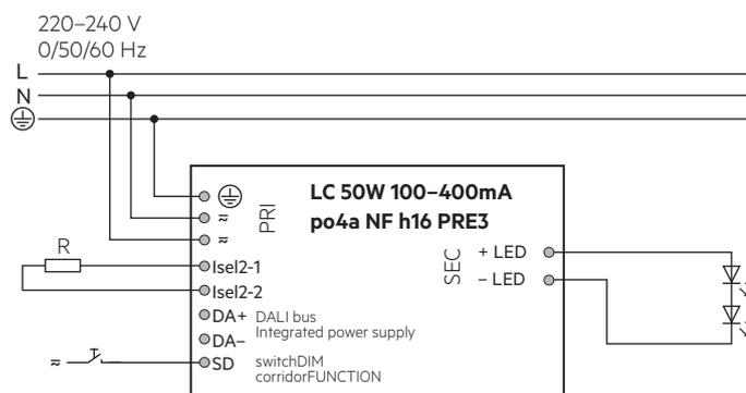
The voltage line for switchDIM / corridorFUNCTION must be the same line as on the mains input of the Driver. In switchDIM applications the DALI interface as well as the integrated DALI bus power supply (IPS) can not be used.
