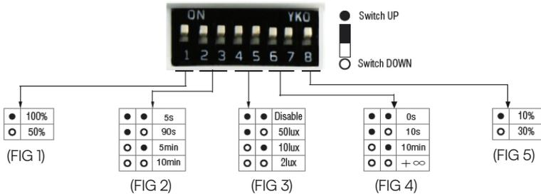
**Detection Area** - It can be adjusted by combining DIP switches for specific application [FIG 1].
