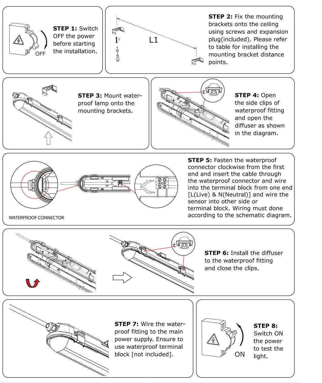
Note: Please refer to the model number and max linkable units which can be linked together. Based on the max linkable units select the max waterproof fittings which you would like to connect.
