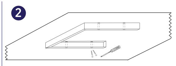
2. Attach the 3 sided U-frame to the ceiling with the screws and holes provided.
