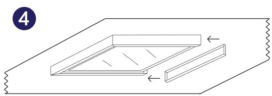
4. Slot the 4th side of the mounting kit to the already attached frame to hold the panel in place.
