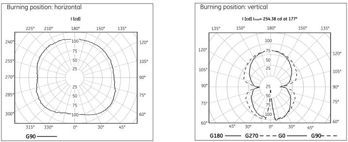
The following diagrams show the polar light intensity distribution of the 2D™ 38W lamp.
