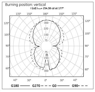
The shape of polar light intensity distribution of the other 2D™ lamps follow the above examples due to the similar lamp shape
