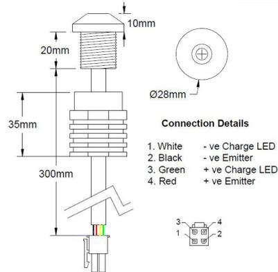
The LED/20/PM/CO is a discrete emergency LED which is designed for panel mount applications along corridors. The bezel has a diameter of 28mm and the cut out required is 20mm.
