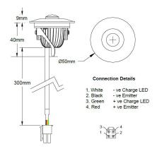
The LED/40/OA is a discrete emergency LED which is designed for ceiling recess applications. The bezel has a diameter of 50mm and the cut out required is 43mm.
