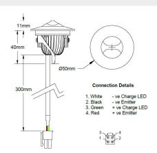
The LED/40/CO/IP54 is a discrete emergency LED which is designed for ceiling recess applications along corridors. The bezel has a diameter of 50mm and the cut out required is 43mm.
