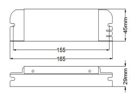
The CBR is supplied either as a changeover module, which can be integrally mounted within the luminaire, or housed in a strain relief enclosure for remote mounting.
