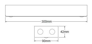
The NED/3/SP98 is supplied as a remote conversion kit for mounting away from the fitting. This kit would be used in applications where space inside the fitting is limited.
