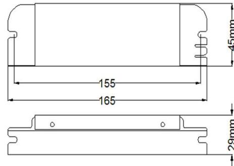
The NES/3 range is supplied as a conversion kit for integral use within a luminaire. If required, it can be provided within a suitable remote enclosure where space inside the fitting is limited.
