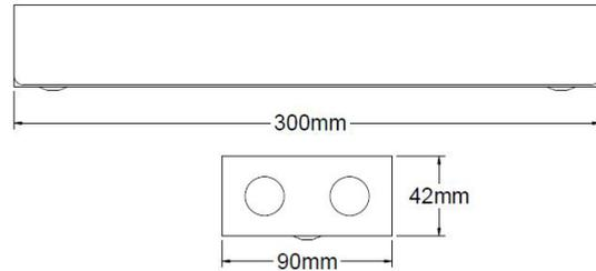
The NES/3/SP98 is supplied as a remote conversion kit for mounting away from the fitting. This kit would be used in applications where space inside the fitting is limited.
