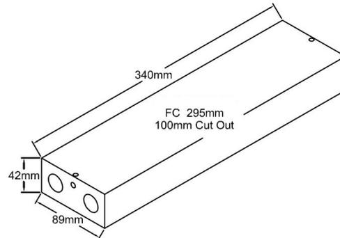
The TED/4/SP100 is supplied as a remote conversion kit for mounting away from the fitting. This kit would be used in applications where space inside the fitting is limited.
