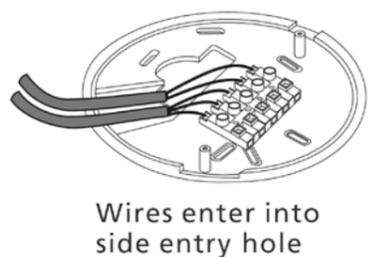
Wires enter into side entry hole
