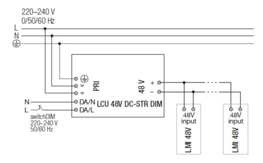
The wiring diagram shows the connection between mains, LCU DC power supply, LMI DC LED Driver.
