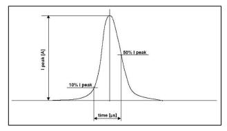
If several control gear are connected to one circuit breaker, the individual inrush currents add up.
