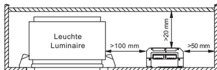
If several ballasts are installed in masts, boxes, etc., measures must be taken to avoid overheating of individual components.
