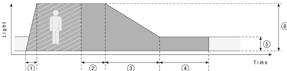
1. Fade-in time: the time that starts as soon as the presence of a person is detected. During the fade-in time the luminous intensity is faded up to the presence value (default: 0s).
