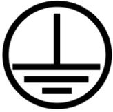
The earth connection is conducted as protection earth (PE). The LED Driver can be earthed via earth terminal or metal housing (if device has metal housing). If the LED Driver will be earthed, protection earth (PE) has to be used. There is no earth connection required for the functionality of the LED Driver. Earth connection is recommended to improve following behaviour.
