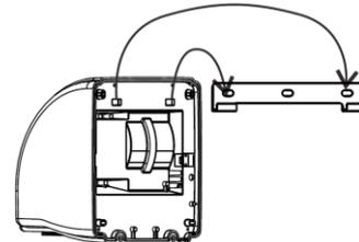
7. Secure the base of the hand dryer using the screws provided
