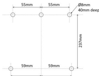
2. Fix the metal bracket to the mounting surface using the wall plugs and the screws provided.
